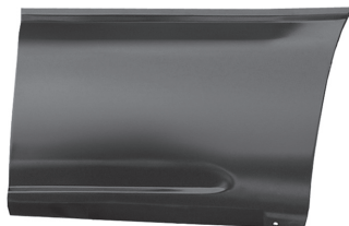
BED: LWR FRT SECT (Left) ..... 0856-143L BED: LWR FRT SECT (Right) ..... 0856-144R 19"H x 27"W, 6'Bed
