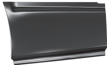
QTRP: LWR RR SECT (Left) ..... 0870-137L QTRP: LWR RR SECT (Right) ..... 0870-138R 18.25"W x 11.5"H, W/O Corner, Blazer
