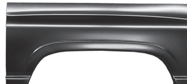
WHL ARCH: UPR SECT (Left) ..... 1582-147L WHL ARCH: UPR SECT (Right) ..... 1582-148R 43"W x 18.5"H
