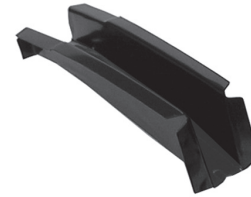
CAB FLOOR: FRT SUPT ..... 0849-309U 4.25"W x 14.5"L, OE Style
