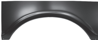
BED: UPR WHL ARCH (Left) ..... 0849-147L BED: UPR WHL ARCH (Right)..... 0849-148R 35.25"W x 14.125"H
